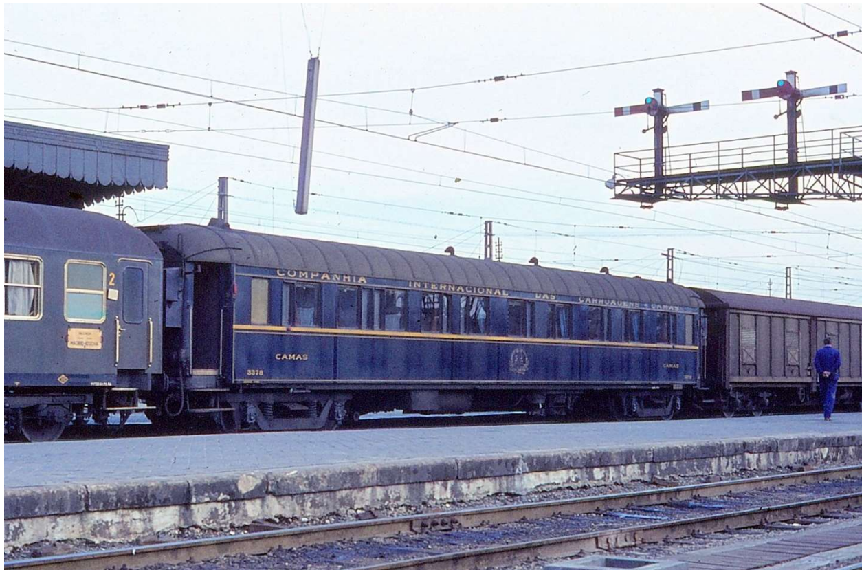
WL 3378, Sleeper of the steel-bodied type S4 (series 3361-3380, Metropolitan 1928)
