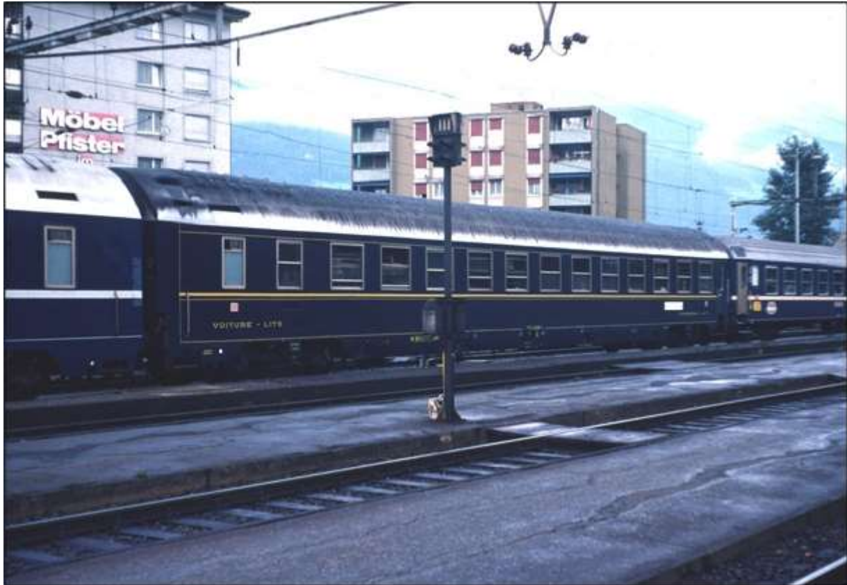
SBB 12-compartment, MU-type Sleeping car in Wagons-Lits markings, on Wiener-Walzer, Sargans, Switzerland (1978/09/07) [PETER DAWES].
