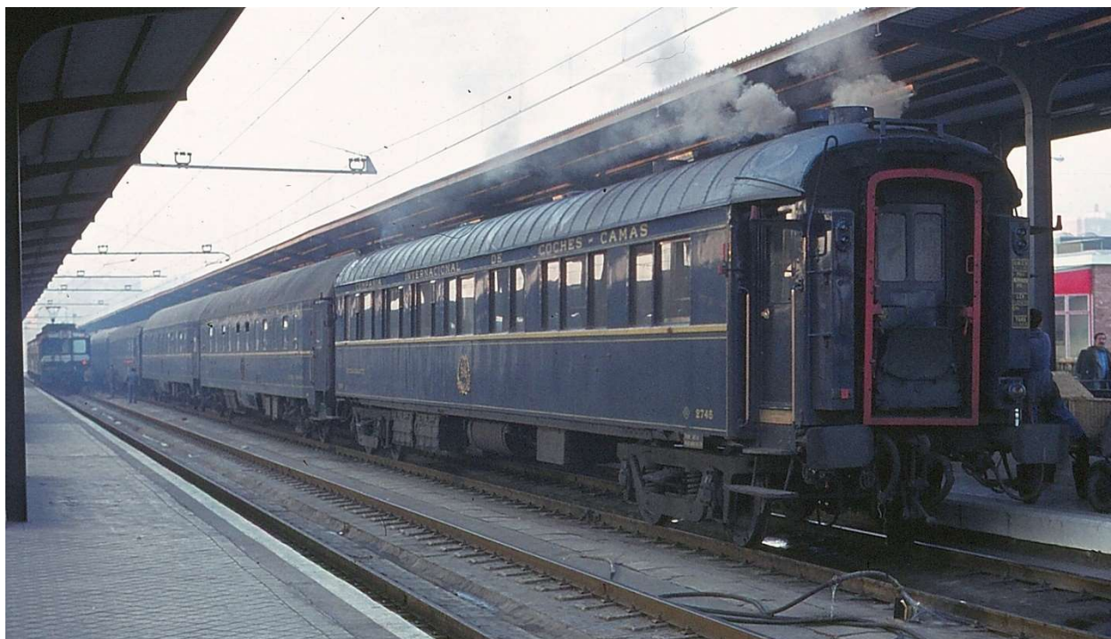
WR 2745 (ex WSPc type „Sud-Express“) on the Puerta del Sol. In front of it, two of the ten UH type sleeping cars converted for Paris-Madrid lane-changing operation can be seen.
