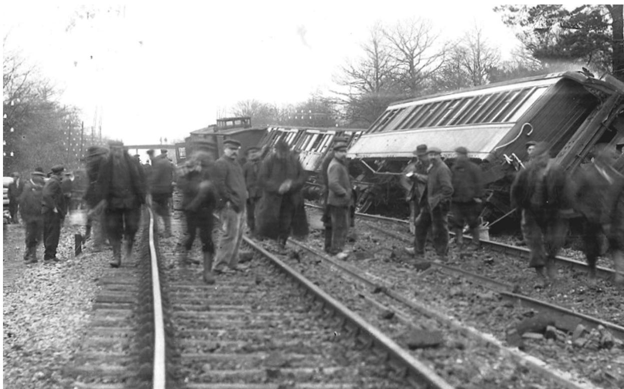
54 Rambouillet Accident. Car 261 was not rebuilt after the accident but had been rebuilt to a Wagon-Restaurant after the Club Train ceased. Note it retains the 17 window arrangement (one filled in) confirming it was originally a 26 seat car. Roland Arzul
