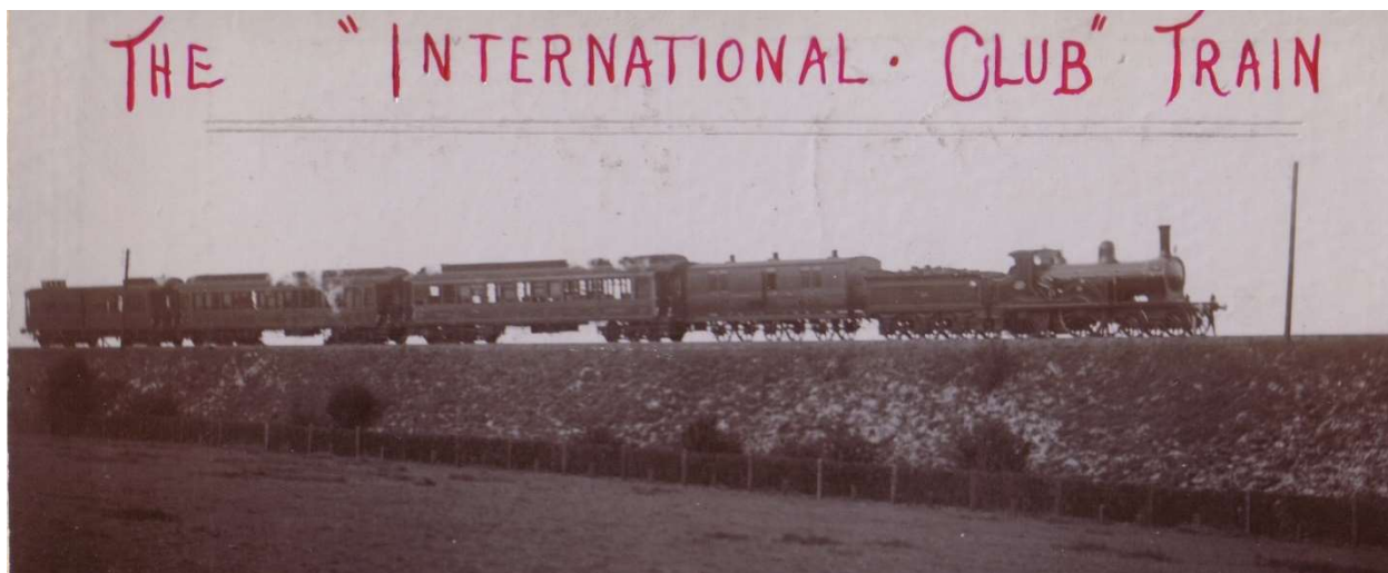
42 This view from early 1893 shows the usual make up of the LCDR train after it had been reduced to two cars. Left to right, Fourgon, 32 seat car, 26 seat car, LCDR 6 wheel brake, Kirtley M3.
