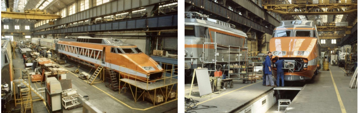
Powerheads of an Alstom TGV Sud-Est in different stages of construction (left) and Power plant of an Alstom TGV Sud-Est under construction, together with a BB.7303 locomotive (right). Photos by the French Railway Society of the United Kingdom. Courtesy Bram Van den Velden.
