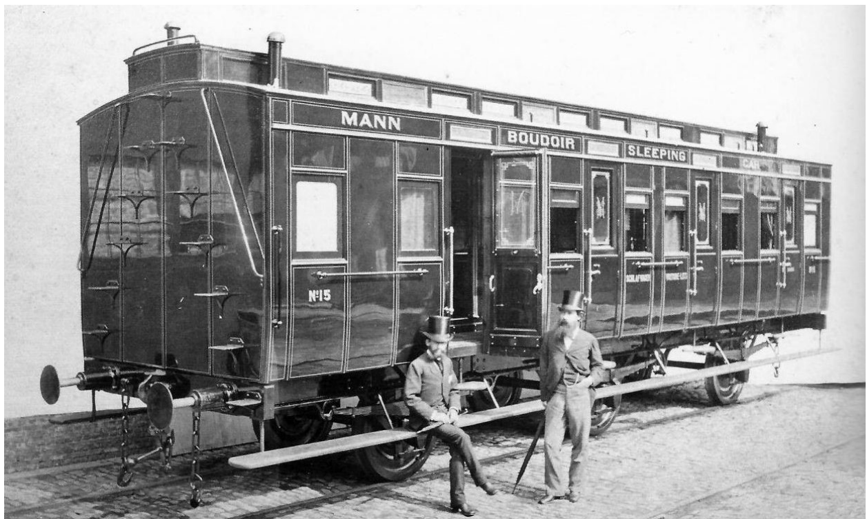
WL No. 15, delivered 1873 from Simmering according to Mann's plans (CIWL/coll. Dirk Frielingsdorf)
