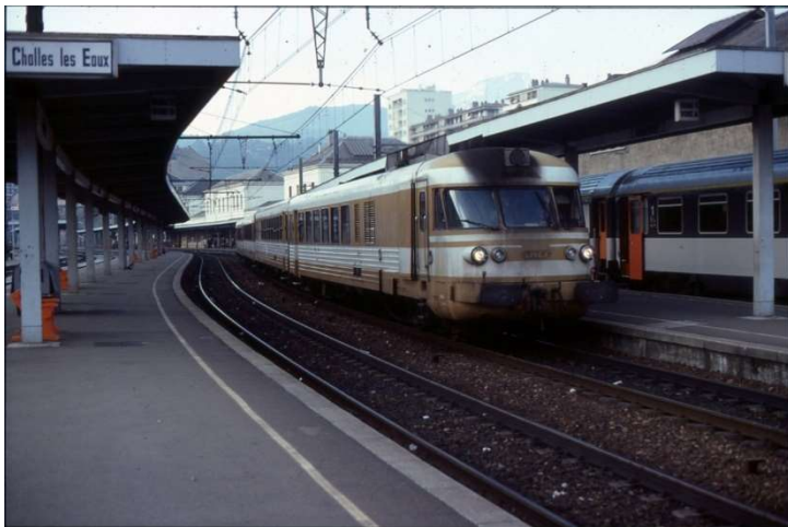
Turbo Train T-1006 belonging to the series T-1001 to T-1014. Chambéry-Challes les Eaux station. August 1, 1980. According to the author of the photo, they were always coupled with the T-1501 to T-1514, which only had a traditional diesel engine. By this time they were assigned to the Lyon depot. Photo Jesús Vigil
