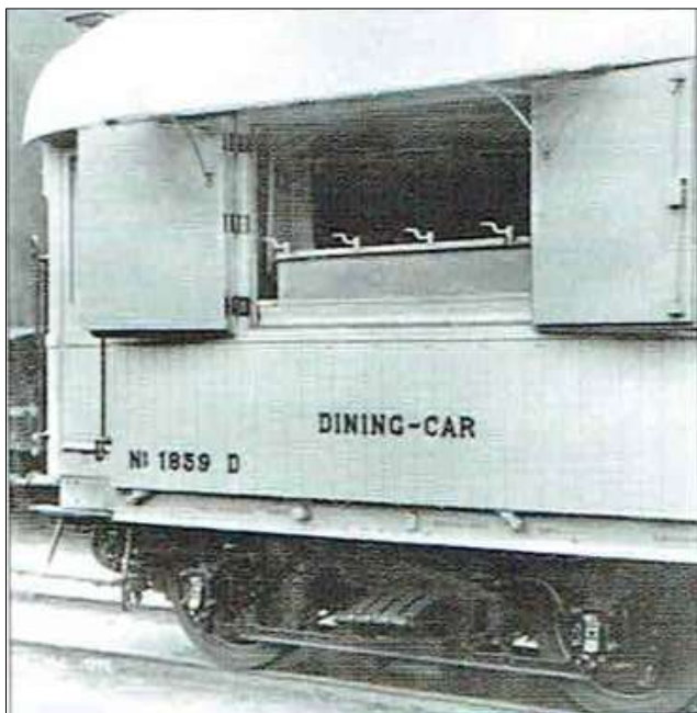
Detail view of ice compartment of dining car no. 1859 opened for filling the container with 400-500 kg of ice Business photo: Ringhoffer / Tatra Collection: Ilie Popescu
