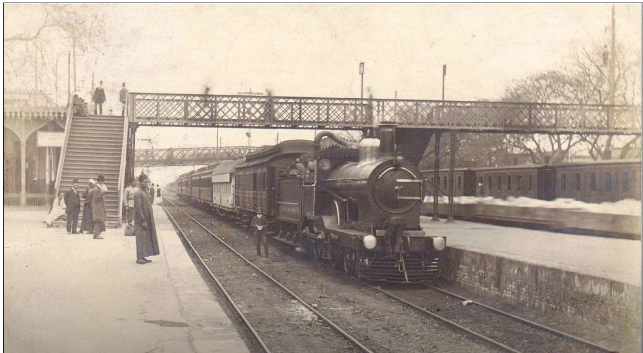
Egyptian State Railways 4-4-0 steam locomotive with a passenger train at Tanta station, 1910's Tanta is situated on the Alexandria-Cairo line Behind the baggage car a white Wagons-Lits car, probably WR 1859 followed by sleeping cars
