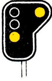
A black rectangular signal with a white border and a white arrow on the right side. It has four circular lights: two yellow lights in the top-left and bottom-left positions, and two white lights in the top-right and middle-left positions. | Passage avec attention; arrêt au signal suivant.        |
