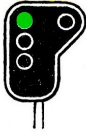
A black rectangular signal with a white border and a white arrow on the right side. It has four circular lights: a green light in the top-left position and three white lights in the top-right, middle-left, and bottom-left positions.       | Passage à ce signal ainsi qu'au signal d'arrêt suivant. |
